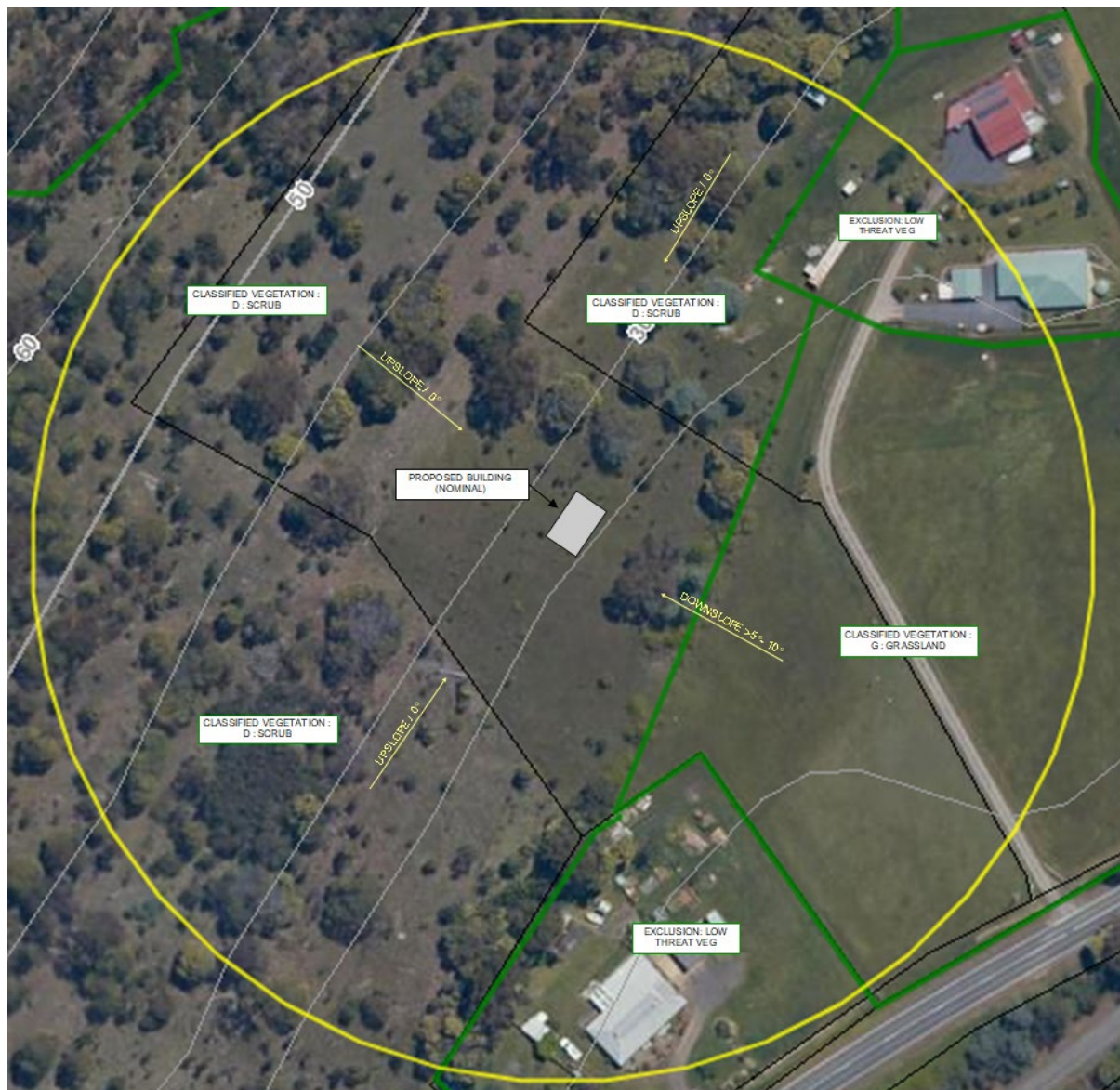
Figure 2: Aerial photo of the area with proposed building area shown. The solid yellow circle is a minimum 100m from edge of the proposed development. Classified vegetation and exclusion shown. Effective slope shown with yellow text and arrows. Source: Land Information System Tasmania, http://www.thelist.tas.gov.au .
