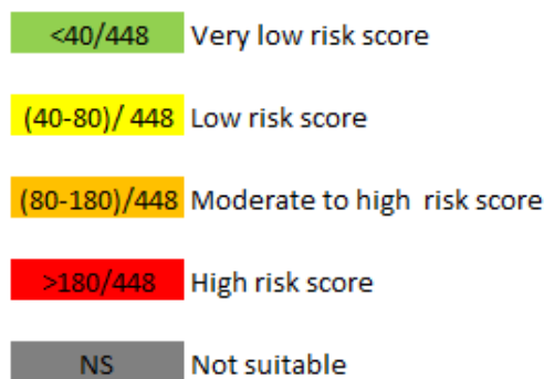
Figure 25 – Austroads Safe System Assessment alignment between crash score and risk
