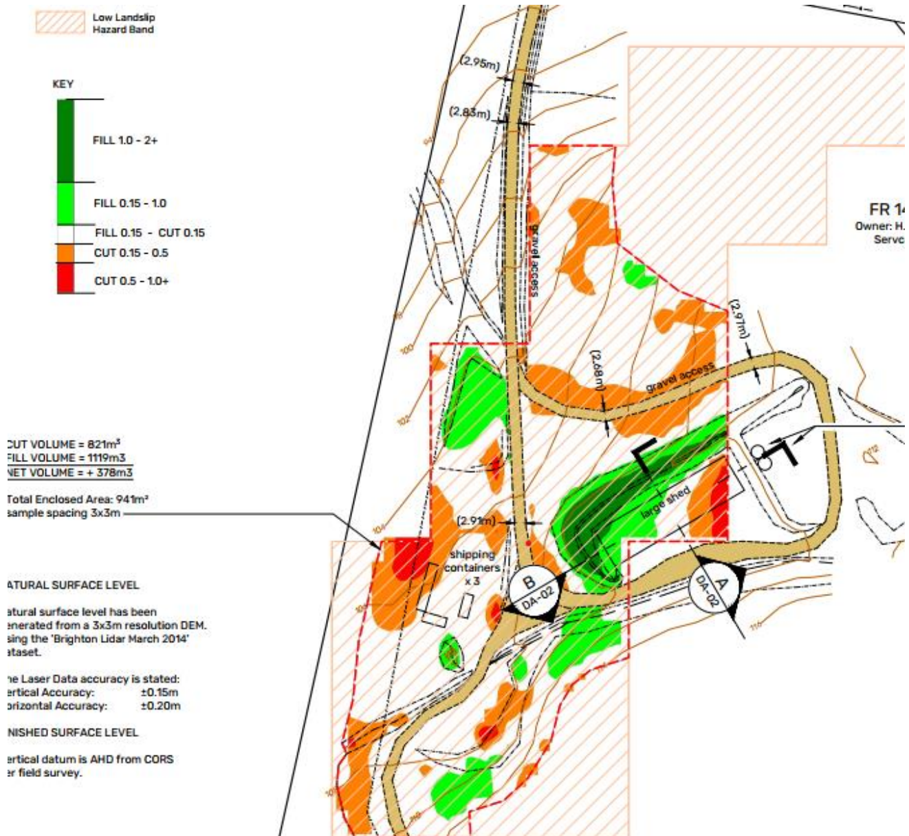
Figure 34: Cut/Fill Plan showing the landslide hazard area with orange diagonal lines (from the application documents).
