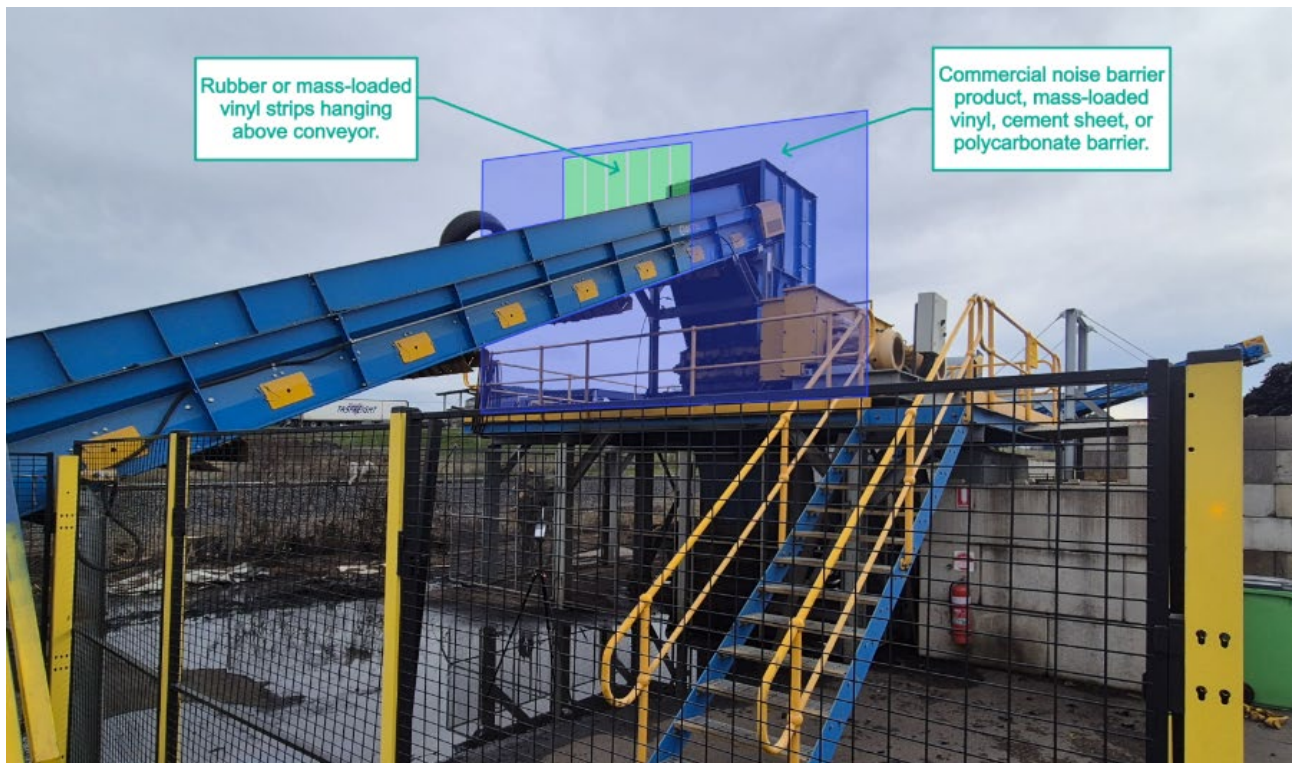
Figure 8 The extent of the proposed acoustic barrier to be installed on the existing shredder. Source: NVC
