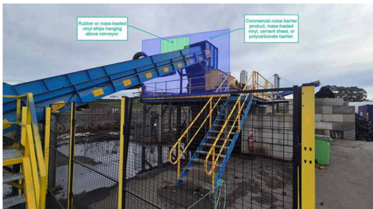
FIGURE 6.1: RECOMMENDED EXISTING SHREDDER BARRIER
