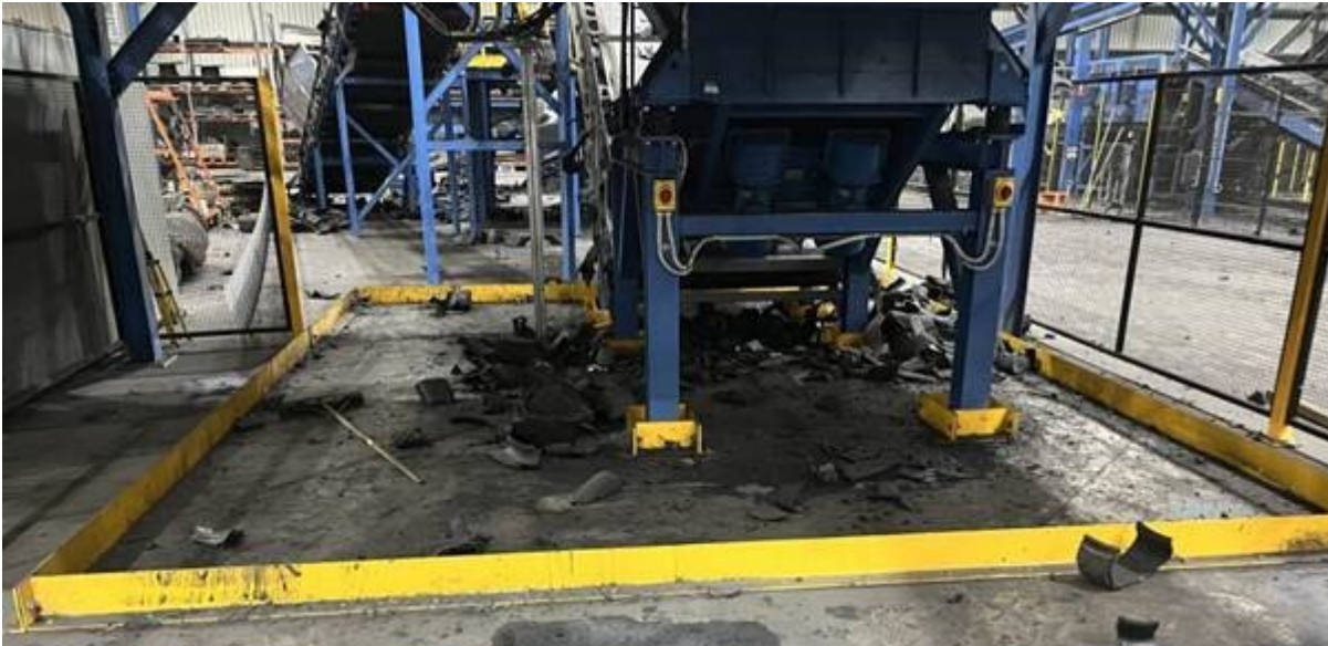
Figure 3-6 Example of proposed shredder bund to be installed under existing and proposed new shredder (Source: Tyrecycle)
