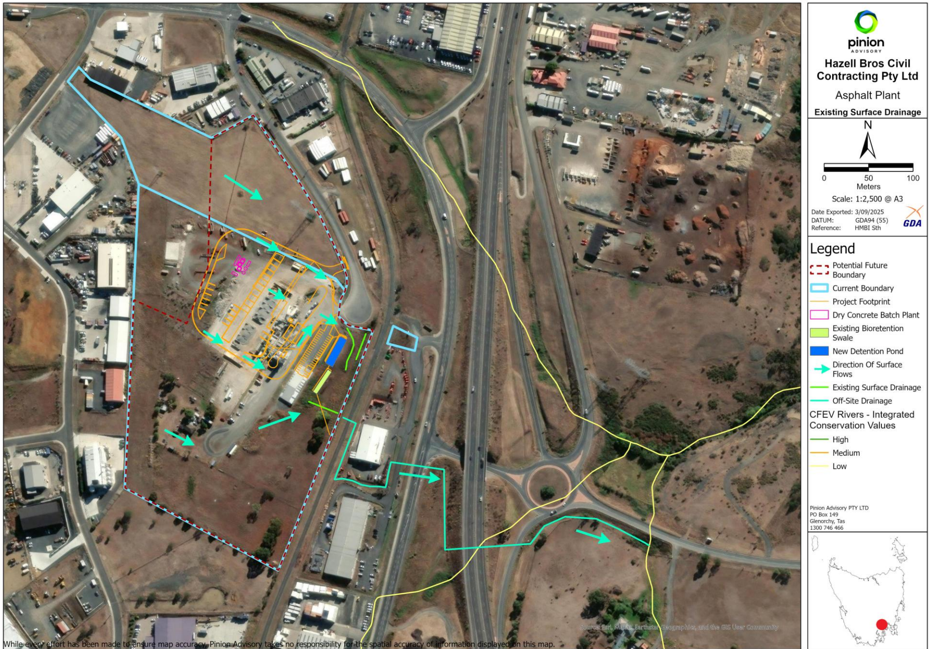
Figure 23. Preferential flow and stormwater drainage from the site
