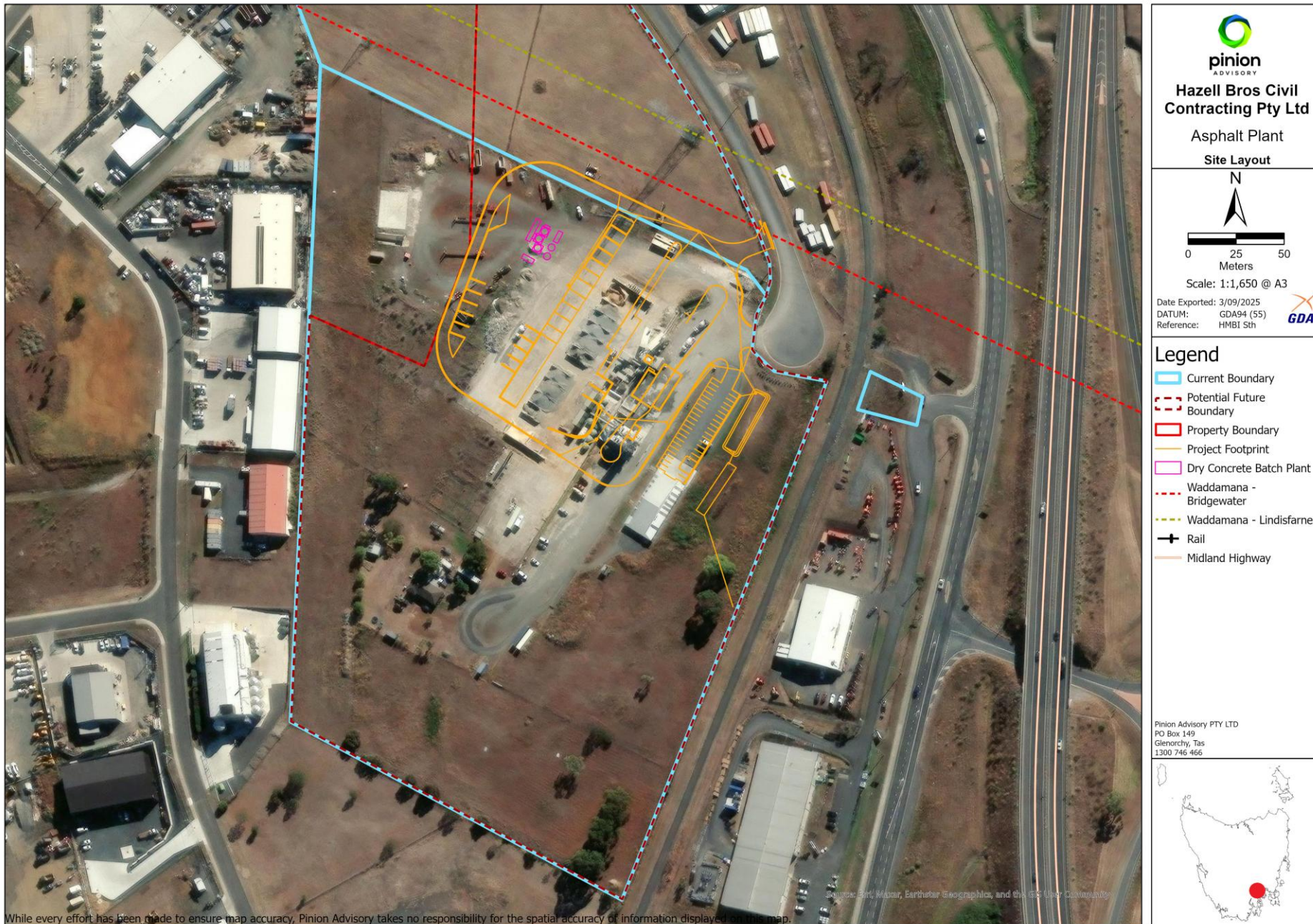
Figure 5. Proposed site footprint showing the proposed asphalt plant (orange line) and relocated concrete plant (pink line)
