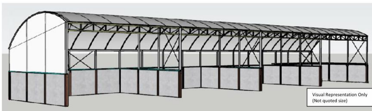
Figure 41. Example of covered storage bays for fine aggregate fractions
