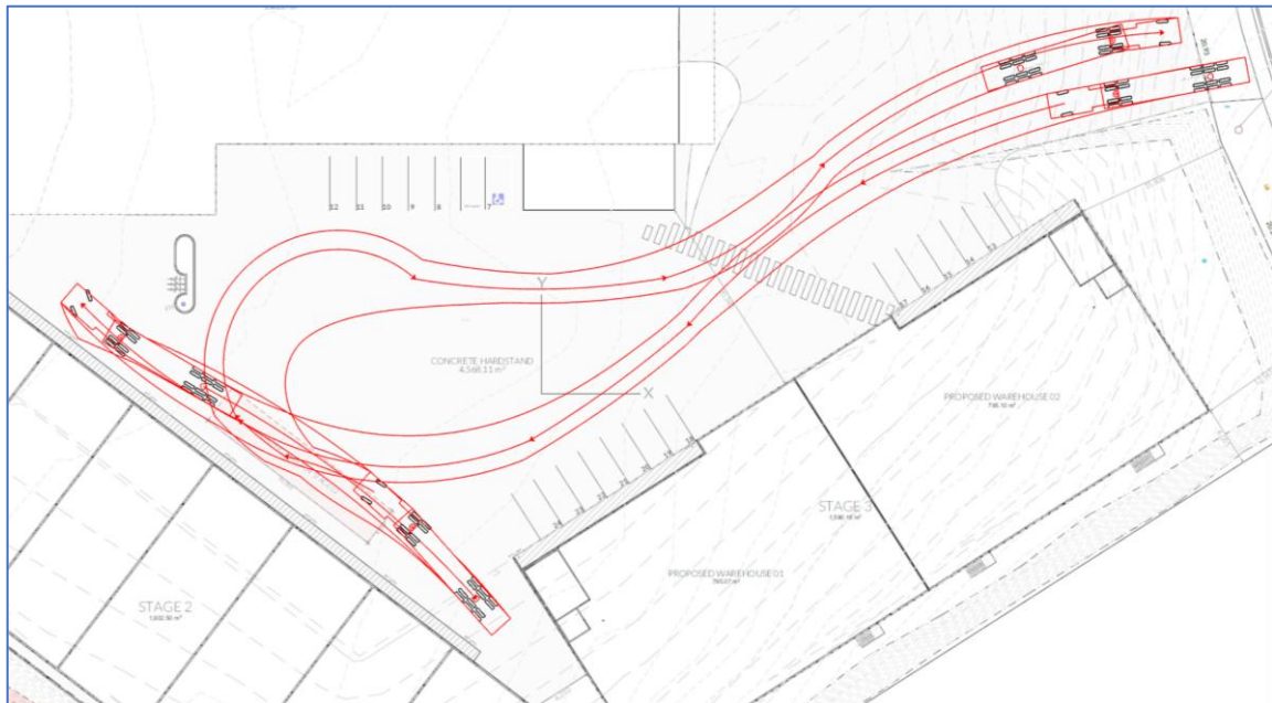
Diagram 8.5 – Swept path of an AV using the designated loading area
