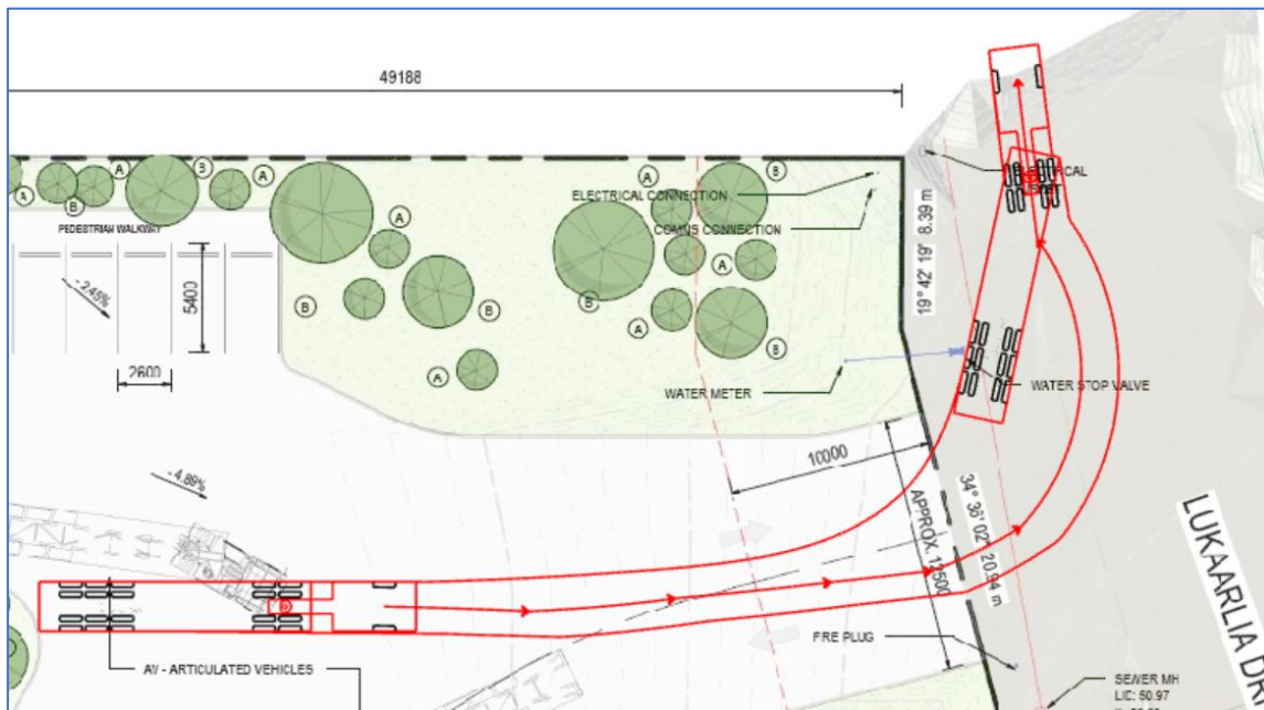
Diagram 13.1 – Swept path of AV turning out of the development site
