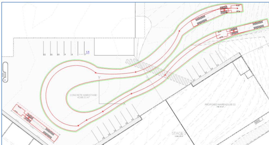
Diagram 8.6B –AV vehicle turning around with a vehicle occupying the designated loading area
