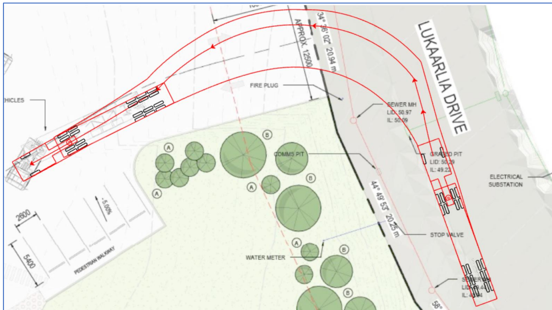
Diagram 13.0 – Swept path of AV turning into the development site
