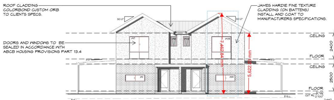
Figure 16 - Typical wall and building heights.
