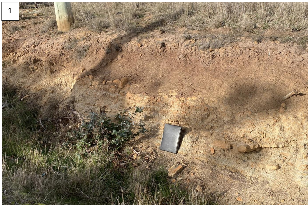
Photo 1: Shallow clay colluvial soil in the upper slopes as reveal in roadside cutting. Clip board is A4. Variably weathered sandy mudstone bedrock at 0.5 – 0.7 m depth
