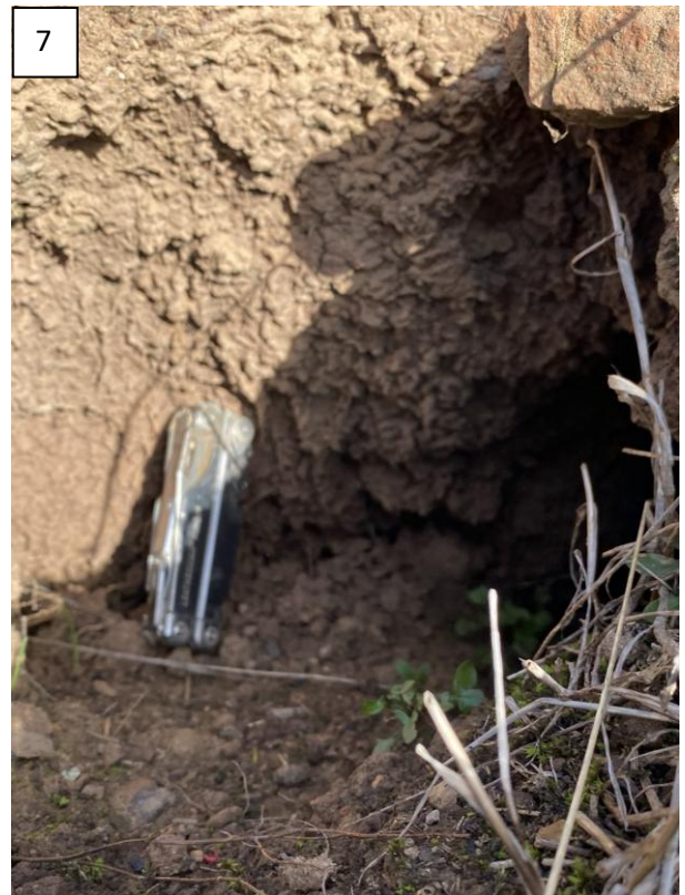
Photos 5-7: Large 'pits' forming tunnel entry points on the eastern slopes on the property. 'Dribble' patterns on the inside walls of the tunnel pits are an indicator of highly to moderately dispersive soil.
