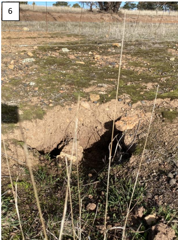
Photos 5-7: Large 'pits' forming tunnel entry points on the eastern slopes on the property. 'Dribble' patterns on the inside walls of the tunnel pits are an indicator of highly to moderately dispersive soil.
