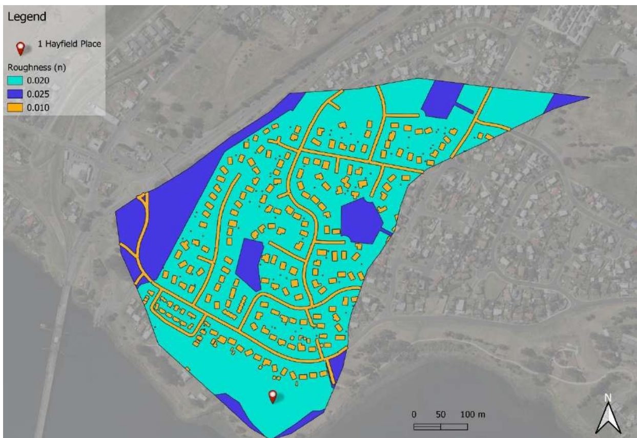
Figure 6. Manning's n derived polygon for the 2D hydraulic model.
