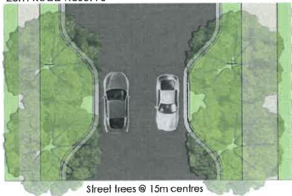
Detail - Collector Road 20m Road Reserve
