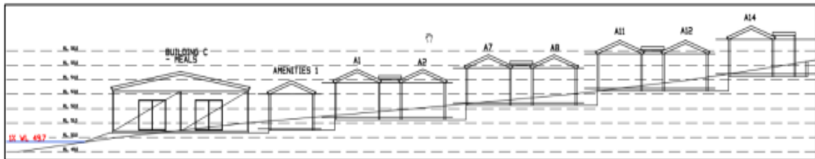
Figure 6. Cross-section through development showing buildings and 1% AEP flood level (PDA Stormwater Report – Revision 3, dated 25 Jan 2024).
