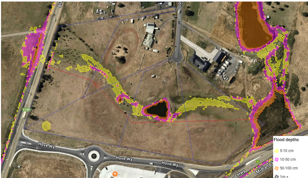
Figure 4. Overland flow mapping for a 1% AEP storm in the Brighton urban area
