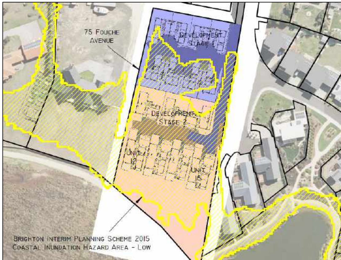
Figure 11. Location of the Coastal Inundation Low Hazard Area in relation to proposed dwellings
