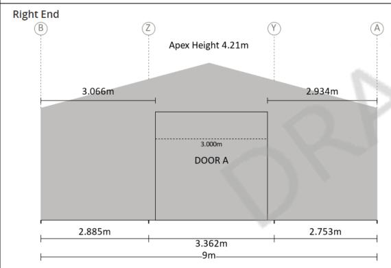
Measurements are from the outside of side girts to the inside of component opening size.
