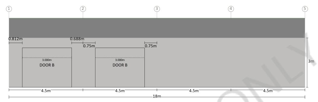
Measurements are from the outside of end girts (end bays) and/or centre of columns (mid bays) to inside of component opening size.
