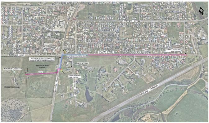
Figure 3 - Proposed sewage connection works (Source: Burbury Consulting)
