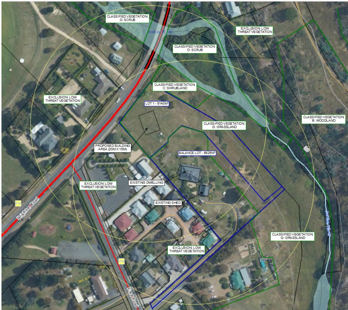
Figure 2: Aerial photo of the area with proposed building area and existing dwelling and outbuildings shown. The yellow circle is a minimum 100m from edge of the proposed building area and existing dwellings. Blue line shows subject lots. Green line shows borders between classified vegetation and exclusions shown. Source: Land Information System Tasmania, http://www.thelist.tas.gov.au .
