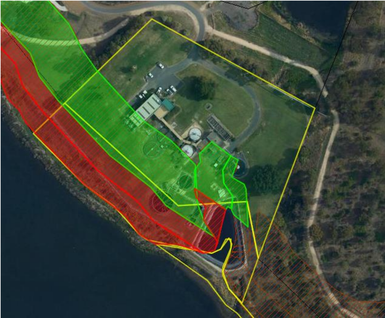
Figure 10: Low band coastal erosion hazard overlay highlighted in green. Medium band coastal erosion hazard overlay highlighted in red. Project site is highlighted in yellow (source: The List, 05.09.2023)
