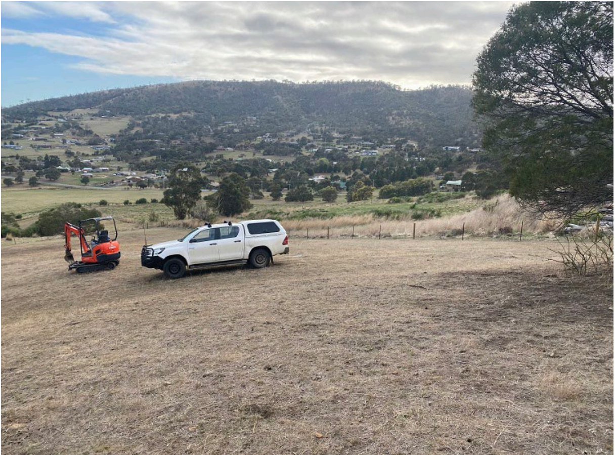
Plates 1 (above) and 2 (below). Views downslope and north-northeast and north respectively across proposed Lot 2. The excavator is at test pit A. The average slope from camera to the lower property boundary is 12°.
