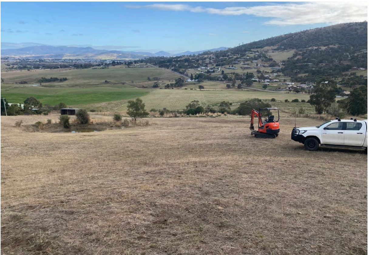
Plates 1 (above) and 2 (below). Views downslope and north-northeast and north respectively across proposed Lot 2. The excavator is at test pit A. The average slope from camera to the lower property boundary is 12°.
