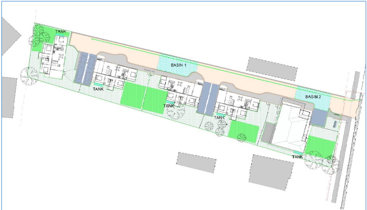
Image 4 – Proposed stormwater onsite detention.
