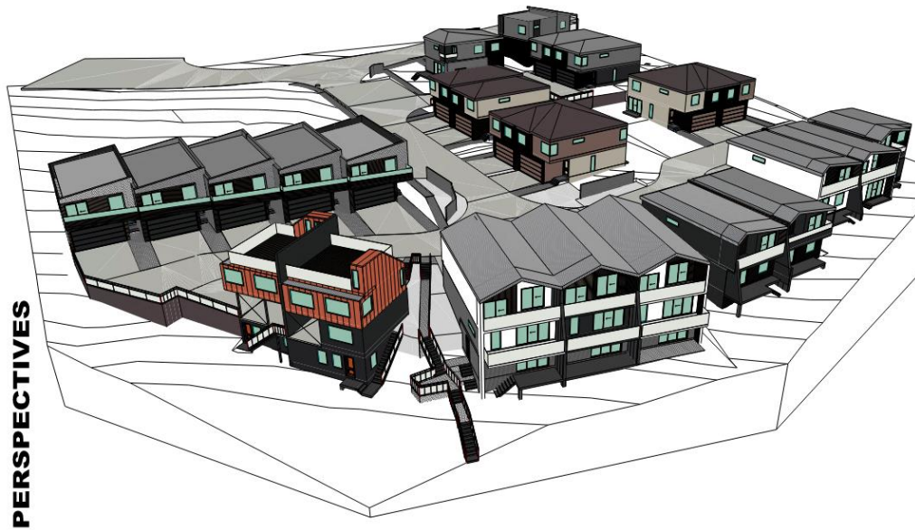
Figure 7 : Perspective view taken from Proposal Documents. Units 16-18 in grey. Units 19 and 20 (timber look, LHS) will be reduced to two storeys (with an approximate height of 6.390m above NGL on southern side)
