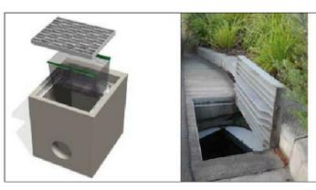
TYPICAL DETAILS OF GRATED PIT LOCATED BEFORE THE LPD (NTS)
