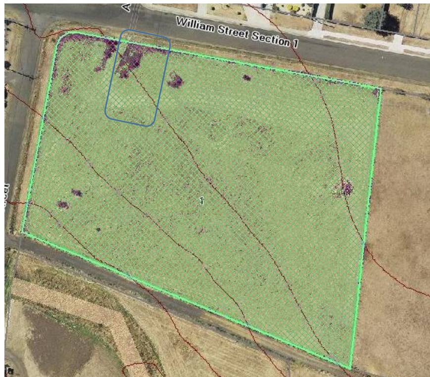
Figure 3: Approximate location of Lot 1 on the site. As shown, the lot fits within the (2m) contours of the land and is generally level (Exponare)
